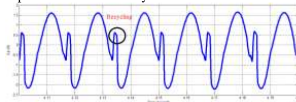
Fig. 13: Waveform of current through the primary of transformer
